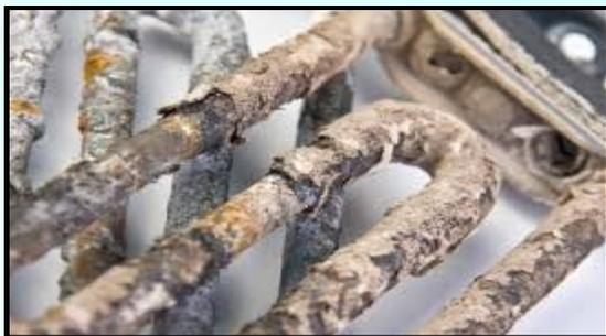
Heating element destroyed with limescale
